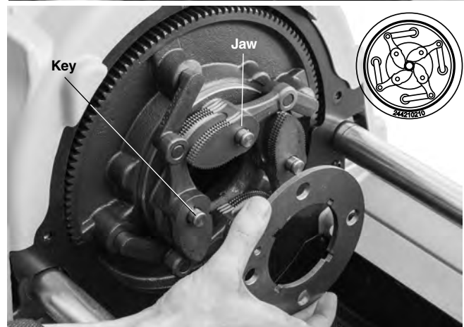
Figure 32 – Changing Auto Chuck Machine Jaws
